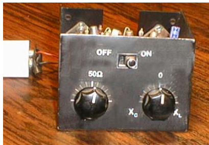
Front Panel with bridge mounted in a simple aluminum chassis
